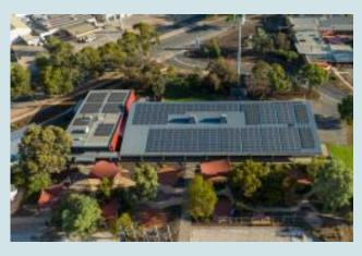
FIGURE 12. 130kw rooftop solar system, Mildura campus
