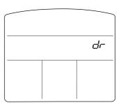
During the drain operation all buttons are in-operative. When the cooler is restarted, there will be a delay while the cooler tank is re-filled with fresh water.
