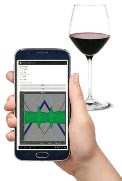
Mobile phone based wine analysis using Fourier Transform AC voltammetry
