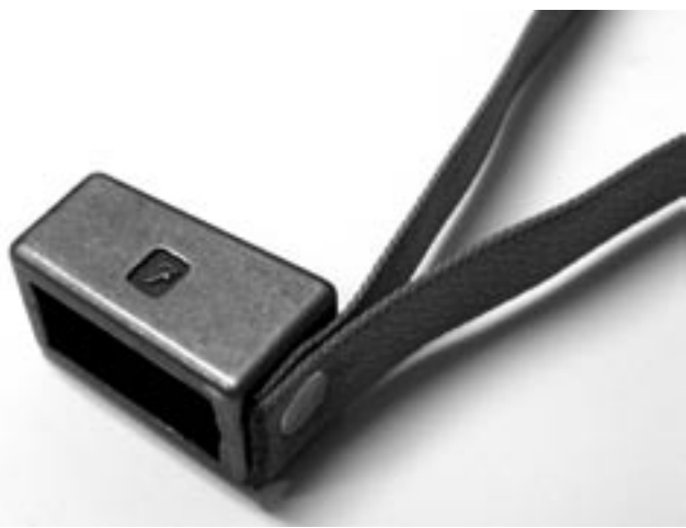
Figure 3: A pull tab made from dacron webbing was riveted to the drop lock to aid in lifting.
