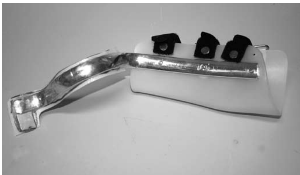
Figure 2: The second version, with a small plate added to the distal end, and a more 'sticky' lining of the aluminium bar.
