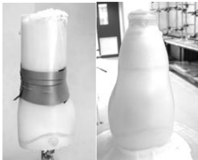
The foamed extension over the original polypropylene mould
