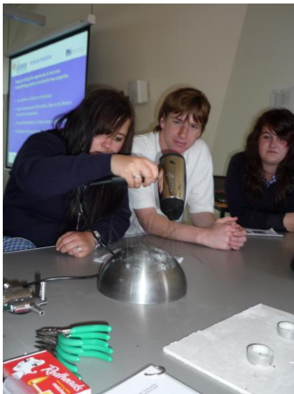
Testing Nitinol with a hair dryer!
