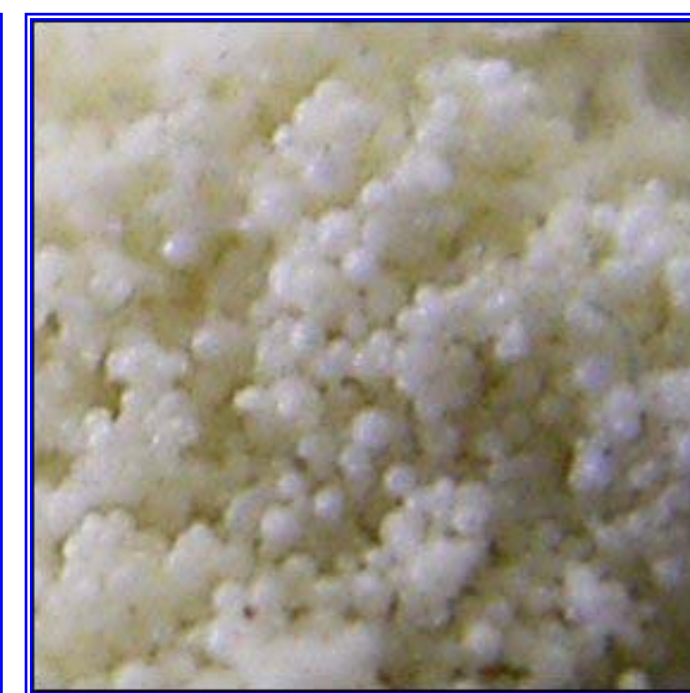
Figure 4. 80%(w/w) PVC & 20% TBP microspheres of 70-150 \mu\text{m} diameter.
